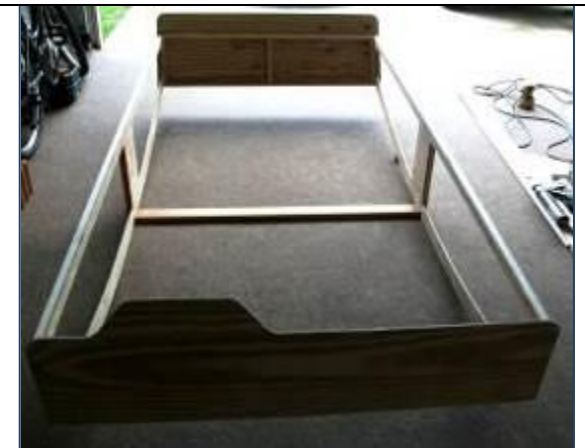
The bow is glued snugly between the inner frame pieces and is aligned along the bottom. The upper cross piece helps support the forward part of the bow deck.
