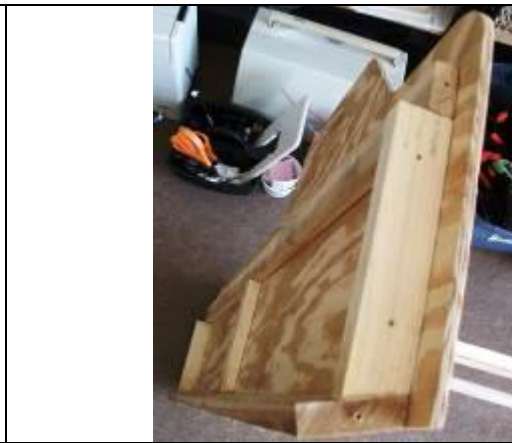
Edge view of the stern transom reinforcing framework. Note the screw holes where the framing will be glued and screwed to the side frame.
