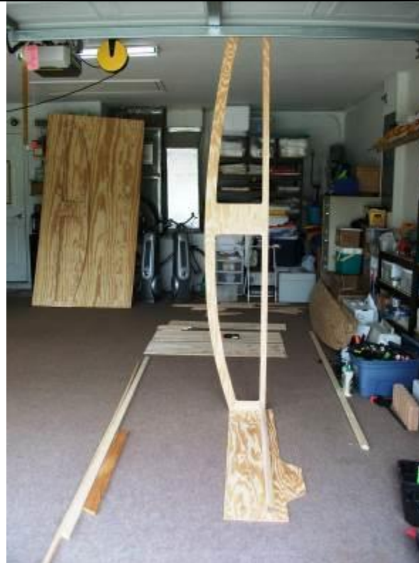
Stand the inside frame on the rear transom to mark where the cross pieces goes. A helper might be needed to hold the frame upright. We follow a similar procedure with the bow framing process. The side frame should be flush with the edge of the stern transom at a width of 47 ½" leaving ¼" on each side of the transom for the sides to overlap.
